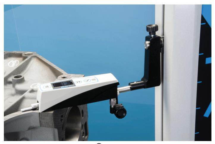
Measuring application for height position with a TESA-HITE measuring column.
