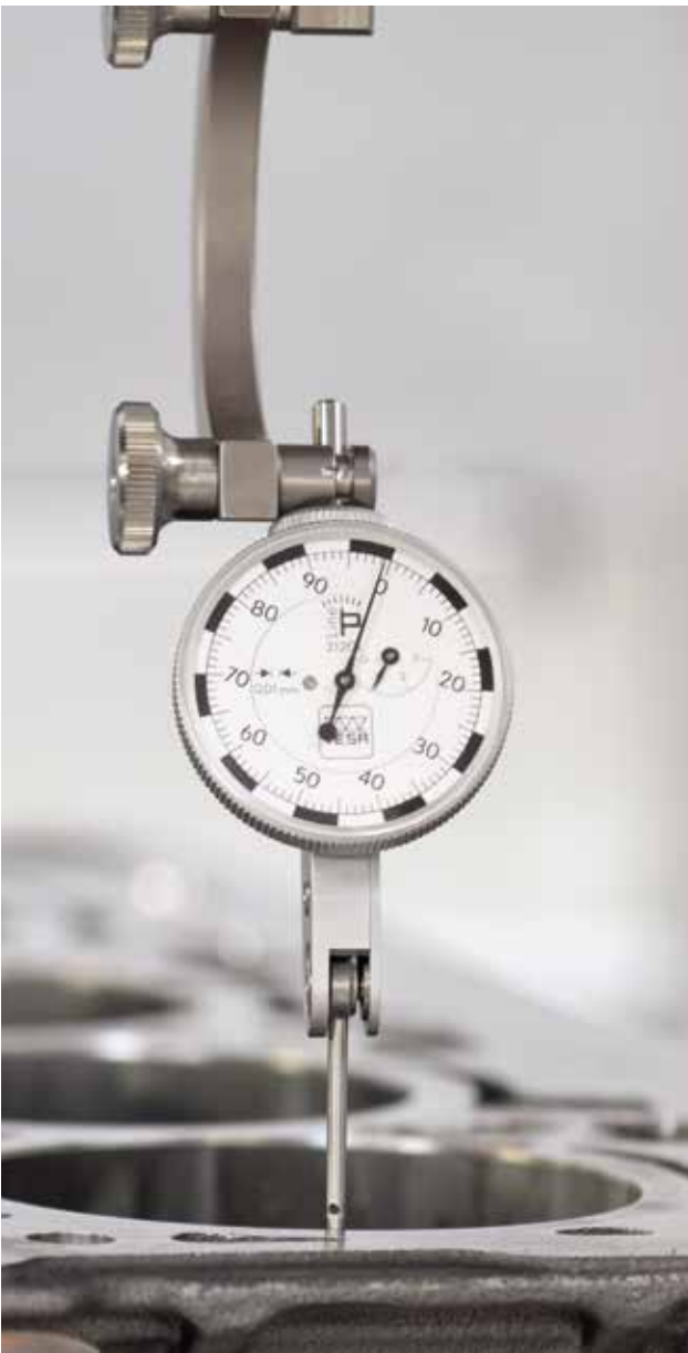
The centering holder allows a large range of movement of the lever-type dial test indicator, useful for measuring at different distances as well as for centering a workpiece on a machine tool.
