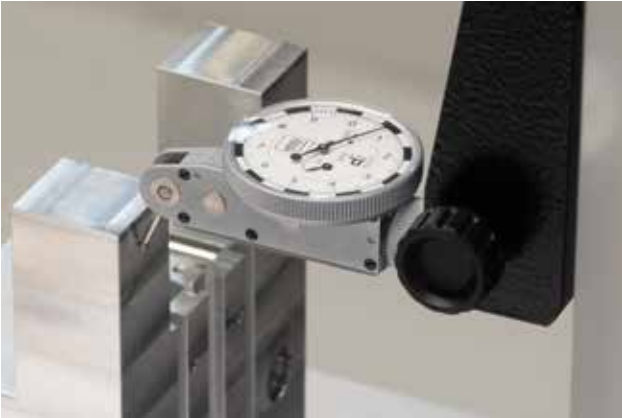
Measurement of the perpendicularity through a P-LINE lever-type dial test indicator mounted on a MICRO-HITE measuring column.
