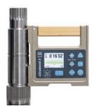
The magnetic measuring faces stabilise the instrument and reduce any influence on the measurement.
