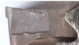
Tool wear after 85 minutes of machining
