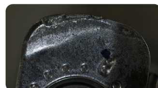
Tool wear after 150 minutes of machining
