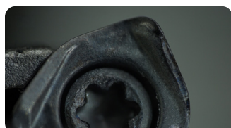
Tool wear after 300 minutes of machining
