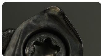
Tool wear after 150 minutes of machining
